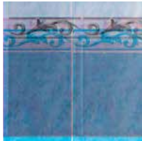
Printing flaws due to irregular belt feed
